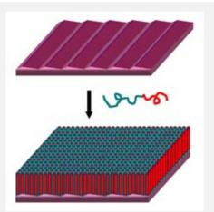
Sawtooth ridges on a sapphire crystal guide the self-assembly of nanoscale elements. Credit: Dong Hyun Lee, UMass Amherst
