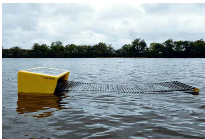
Figure 5.14. “Seaswarm” is a nanotechnology-enabled oil-spill-cleaning robot developed by a group of MIT engineers ( TechNews Daily , August 25, 2010). The conveyor belt of the robot is coated with a mesh of superhydrophobic nanowires developed by Stellaci and coworkers (2008).
