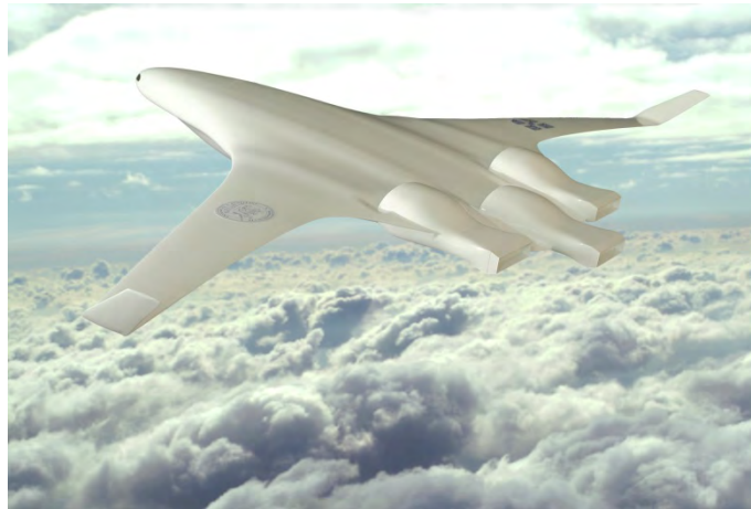
Figure 11.11. Nanotechnology will be used extensively in future aircraft designs including this blended wing body subsonic aircraft (courtesy of Michael Meador, NASA).
