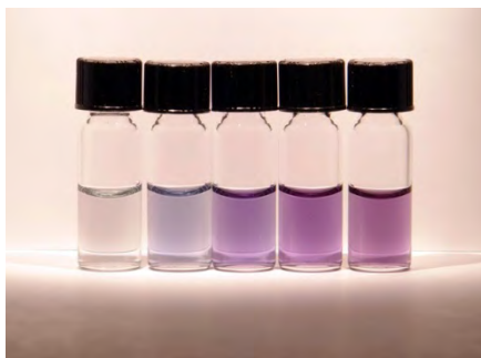
Figure 11.9. Following DGU and subsequent fractionation, optically pure SWNT samples are isolated into distinct cuvettes. The color differences between these vials provide clear visual evidence for the success of the DGU process in sorting SWNTs by their physical and electronic structure (courtesy of Mark Hersam, Northwestern University).
