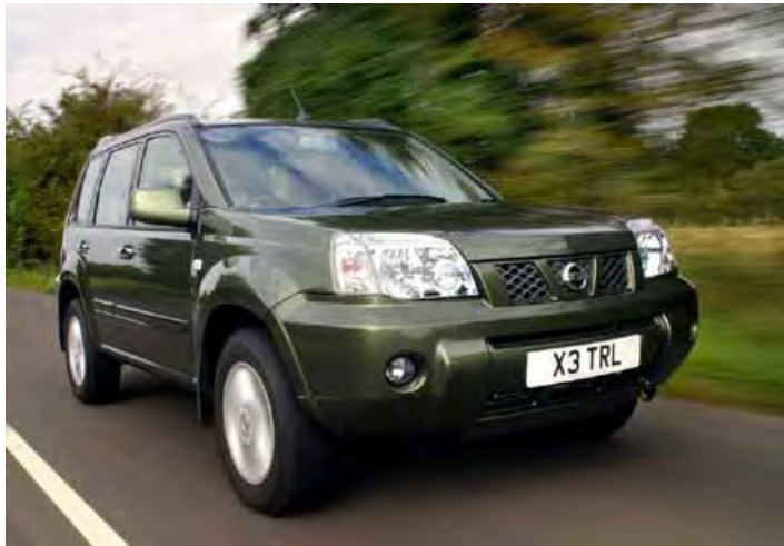
Nissan's X-Trail SUV has CNT-reinforced bumpers
