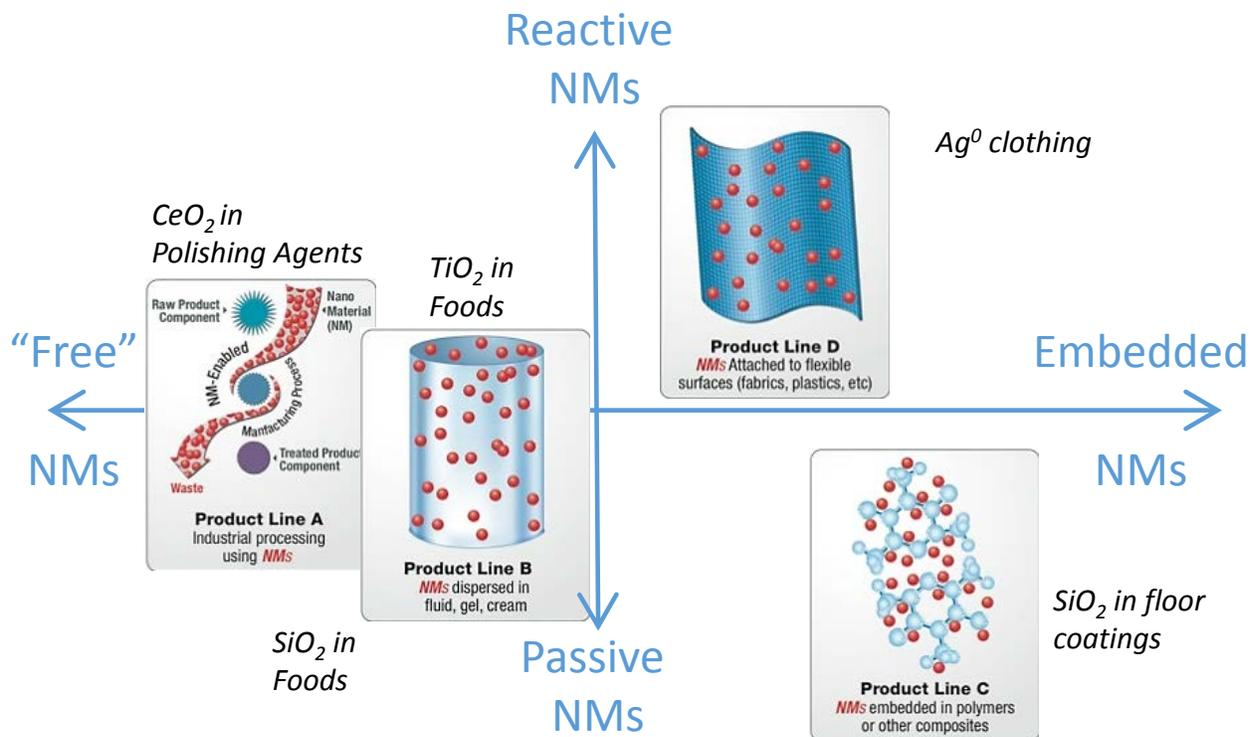
**Figure 2.1. A proposed framework for binning nanomaterials.** The framework organizes nanomaterials along two dimensions: (1) whether they are active or passive, and (2) whether they are freely dispersed or embedded. (Source: P. Westerhoff.)
