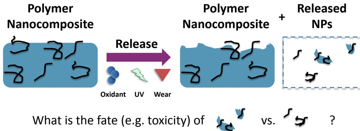
**Figure 5.1** Concept of carbon nanotubes released from polymer nanocomposite. (Source: H. Fairbrother.)
