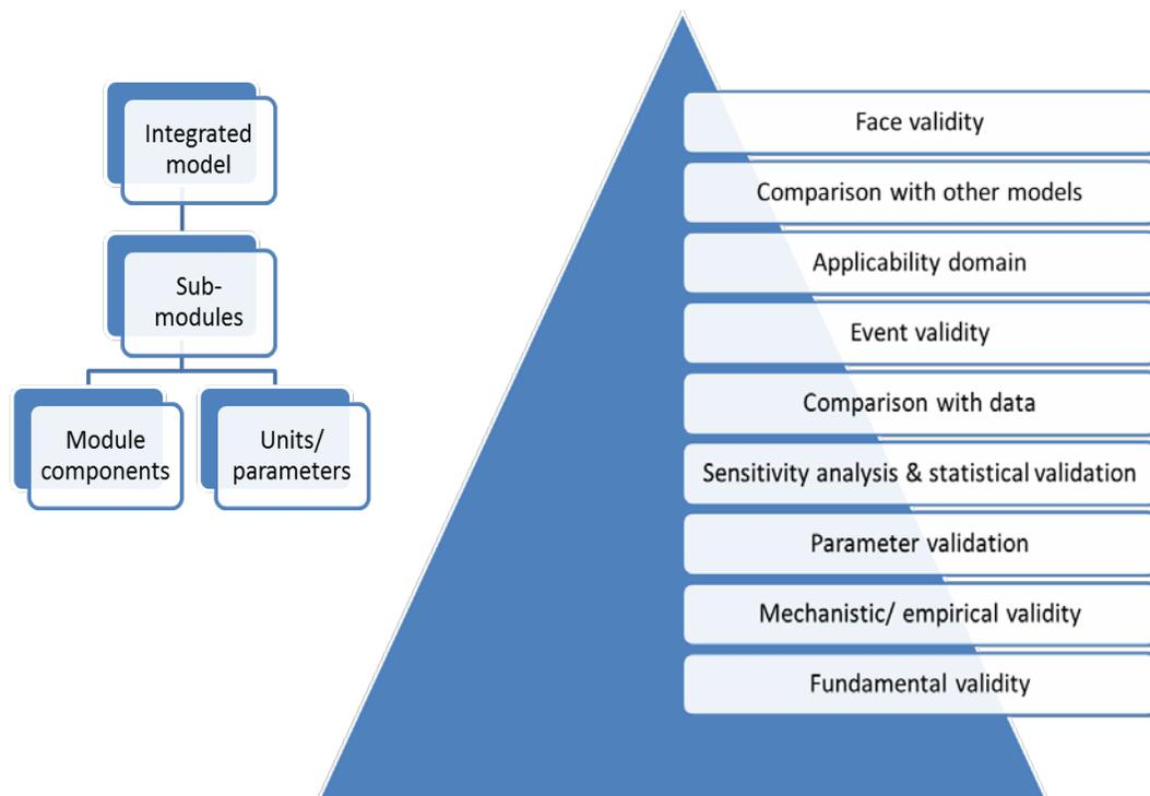
**Figure 4.3. Model validation framework.** Model validation can be accomplished for various model components (left) and for the different model steps (right) where the steps are progressively more significant toward the base of the model validation pyramid. (Source: Y. Cohen.)
