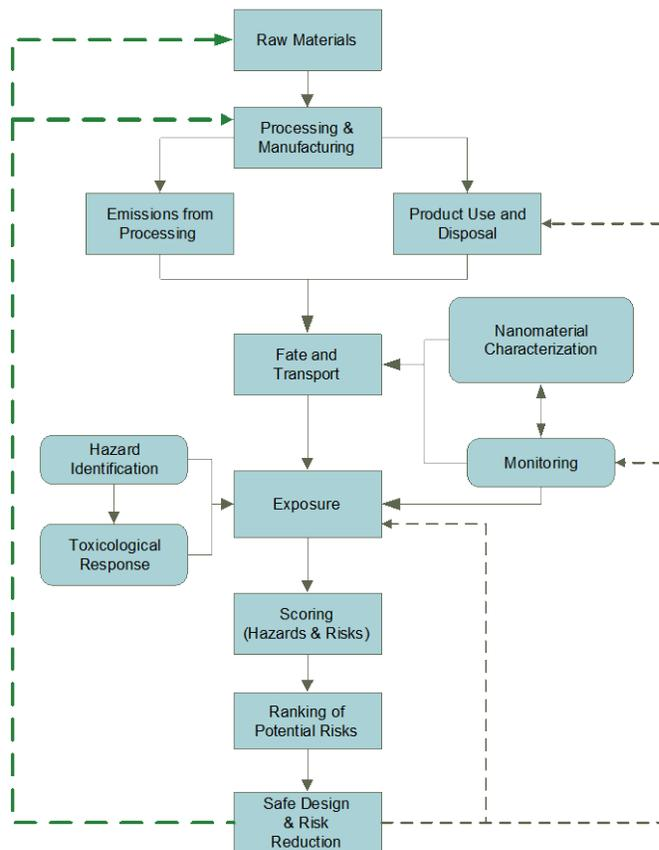
**Figure 4.2. Potential process for analysis and identification of risk management options geared throughout the ENM life cycle.** In this approach the hazard and risk analyses are direct inputs into the decision process regarding action that may be taken (dashed arrows) to change manufacturing processes, provide guidance or regulatory action with respect to product use and disposal, as well as identify the need for monitoring and material characterization. (Source: Y. Cohen.)
