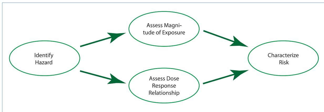
**Figure 1.1. Risk assessment process.** The risk assessment process is often defined as a mathematical equation, Risk equals Hazard times Exposure, or  $R = H \times E$ , and indicates that the magnitude of the risk is equal to the magnitude of the hazard measurement (dose-response) made for a material multiplied by the magnitude of the exposure. (Source: U.S. EPA.)
