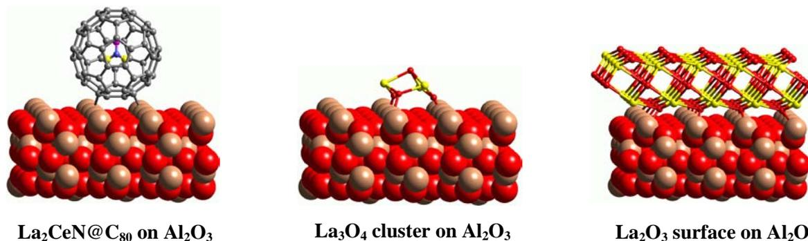
*Schematic of novel molecular and nanometer lanthana catalytic materials for potential application in the activation and functionalization for a range of hydrocarbon intermediates. Left: La<sub>2</sub>CeN encapsulated endohedral fullerene cages supported on alumina. Middle: Supported molecular La<sub>x</sub>O<sub>y</sub> complexes. Right: Nanometer La<sub>2</sub>O<sub>3</sub> thin films supported on alumina (figures courtesy of M. Neurock, University of Virginia, and H. Dorn, Virginia Tech).*
