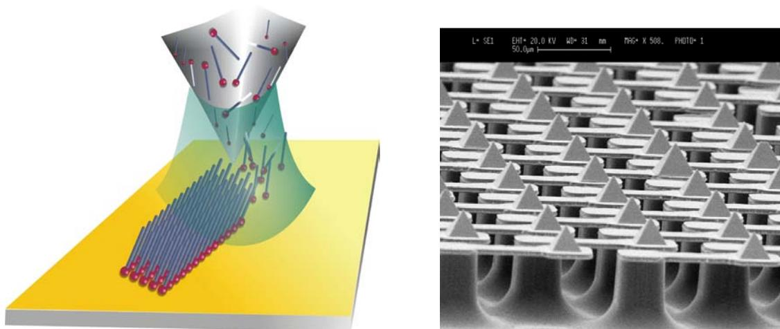
*Left: Schematic illustration demonstrating the concept behind dip pen lithography. Right: A portion of a 10,000-pen array used for doing massively parallel dip pen nanolithography (images courtesy of Prof. C. Mirkin, Northwestern University).*
