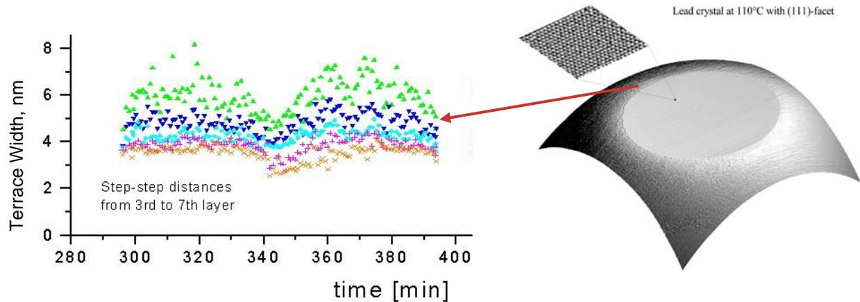
*Example of structural fluctuations in the nanoscale features of a micrometer-scale lead crystallite as it approaches its equilibrium shape. The terraces bounding the edge of the crystallite fluctuate with increasing amplitude until just before the nucleation of a new shrinking layer occurs at ~340 minutes (figures courtesy of K. Thürmer, Sandia National Laboratories).*
