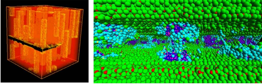
*Left panel: Simulation of fractured silicon nitride (red) ceramic reinforced with silica-coated silicon carbide fibers (yellow). Right panel: Close-up of the fractured composite system. Small spheres represent silicon atoms and large spheres represent nitrogen (green), carbon (magenta), and oxygen (cyan) atoms (figures courtesy of R. K. Kalia, A. Nakano, and P. Vashishta, University of Southern California).*
