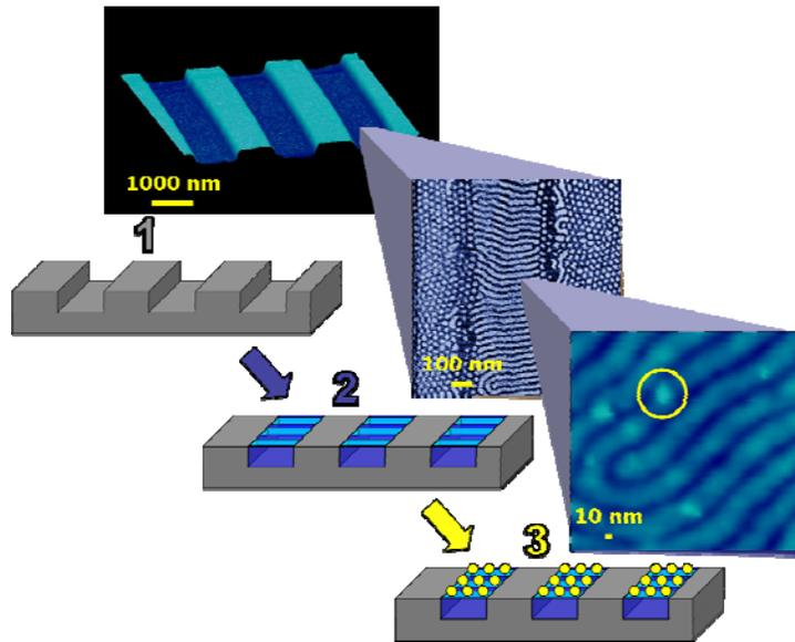
**Stage 1:** Substrate with lithographically prepared trenches
