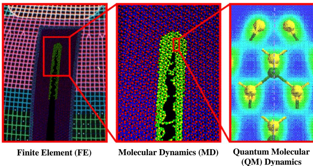
*Schematic of hybrid multiscale finite element/molecular dynamics/quantum mechanical simulation of fracture. Continuum FE simulation invokes MD simulation near the crack tip and fractured surfaces to describe atomistic processes, which in turn invokes QM simulation at the crack tip to handle bond breakage/formation and chemical reactions involving environmental molecules (images courtesy of P. Vashishta, University of Southern California).*
