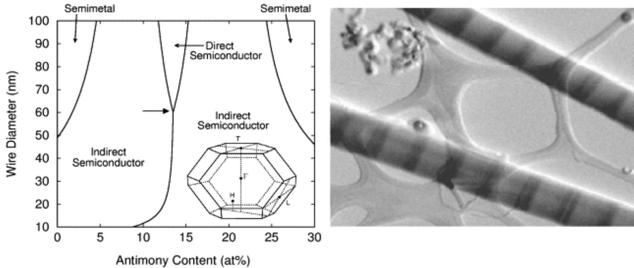
Left: Variation in electronic structure of Bi-Sb nanowires as functions of composition and wire diameter (image from Lin *et al.*, Proceedings of the 21<sup>st</sup> International Conference on Thermoelectronics, 253; reprinted with permission, © 2002, IEEE). Right: Superlattice Ge/Si nanowire (image adapted from Li *et al.*, Appl. Phys. Lett. 83, 3186; reprinted with permission, © 2003, American Institute of Physics).
