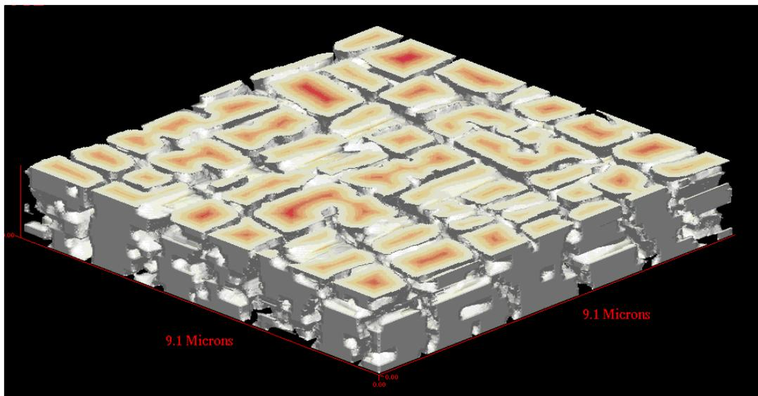
*Focused ion beam tomography is used to reconstruct the internal cellular temperature of a high temperature Ni-based super alloy with a spatial resolution of order 10 nanometers (image courtesy of A. Kubis, D. Dunn, R. Hull, UVa, and D. Bachmann, GE).*
