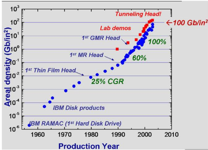
Top left: Evolution of hard drive storage capacity vs. year first in production (image courtesy of S. Parkin, IBM). Bottom left: Schematic image of a magnetic disc drive. Bottom right: Atomistic simulations of a giant magnetoresistive layer structure (image from X. Zhou et al., *Acta Mater.* **49**, 4005 (2001); reprinted with permission from Elsevier).
