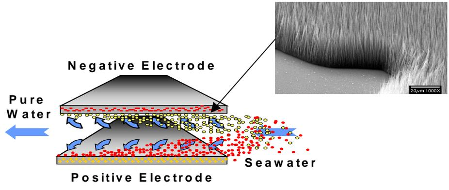
High surface area, high-conductivity electrodes from aligned carbon nanotubes
