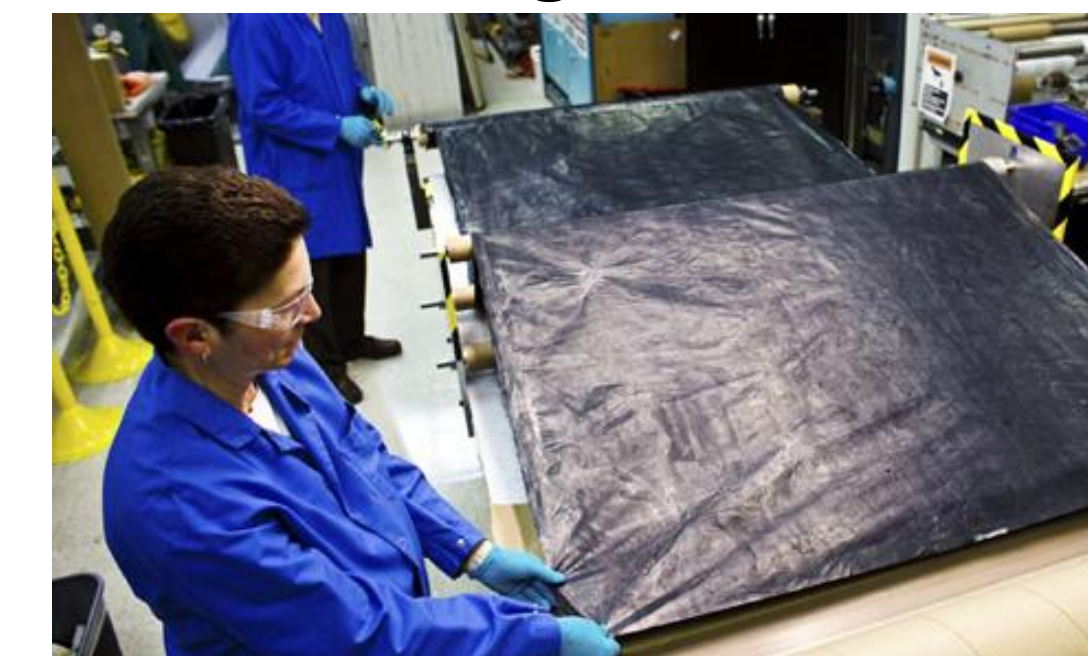
Workers glue sheets of carbon nanotubes together with an industrial adhesive. This sheet is 61 meters long (Courtesy of MIT).
