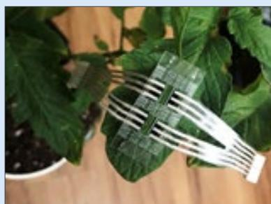
The flexible sensor continuously monitors plants to detect stresses and diseases. Image credit: North Carolina State University.
