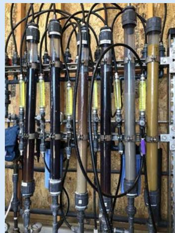
Column filtration system at the Orange County Water District pilot test; the far left column contains the adsorbent. Image credit: Cyclopure.
