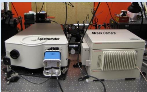
The spectrometer (left) and streak camera (right) funded by DURIP that enabled researchers to study atomically thin materials. Image credit: Marko Loncar, Harvard University.
