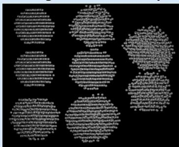
3D images of platinum particles between 2–3 nanometers in diameter in liquid under an electron microscope. Image credit: Peter Ercius, Berkeley Lab.
