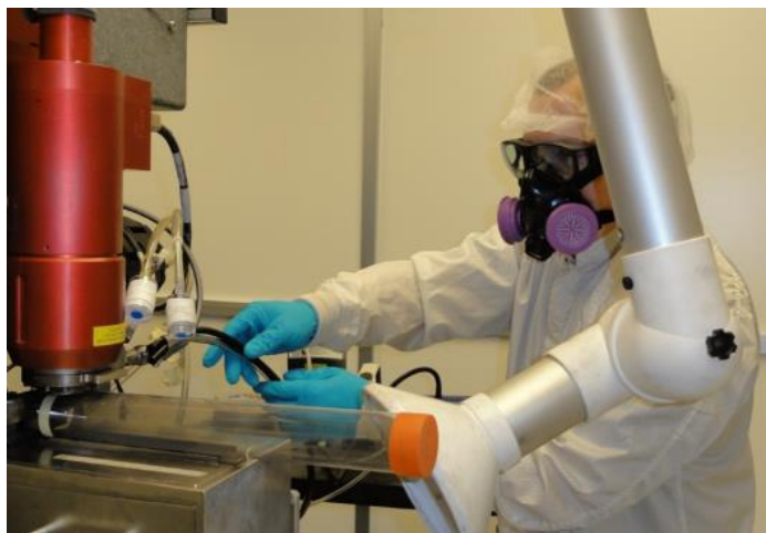
Figure 2. Nanomaterial workplace assessment. Here a NIOSH field team member sets up integrated filter-based samples that are used to confirm the presence of nanoparticles. Image credit: NIOSH ( www.cdc/niosh-science-blog/category/nanotechnology ).
