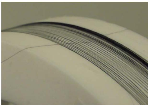
**Figure 3.** Image of wet-spun carbon nanotube fibers. The fibers on the drum are bundles of several fiber filaments with each filament having a diameter of approximately 25 micrometers (source: Rice University).
