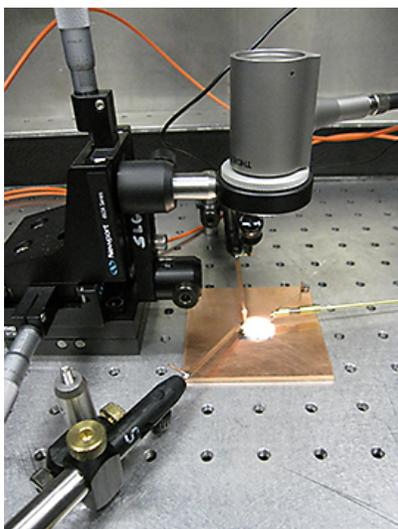
**Figure 2. NIST Super-Continuum Laser Solar Simulator. (Source: NIST)**
