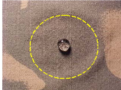
Normal Lighting, Outer Face (yellow indicates wet area on inside) (drop rolled slightly to right)
