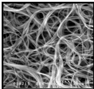
Figure 1. Single wall carbon nanotubes created by laser ablation at RIT
