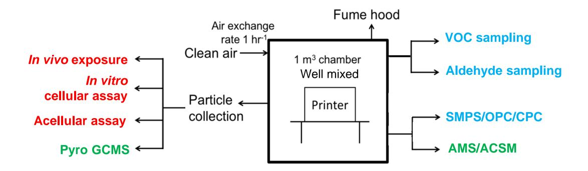
Test procedures and emission calculations follow basis of RAL-UZ 205 Blue Angel Method (BAM) developed for laser printers.
