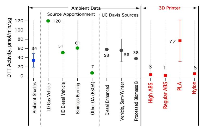
ABS and Nylon particles similar to lowest levels of ambient sources (biogenic emissions) PLA similar to vehicle (gas and diesel) and biomass burning (wood smoke) by DTT assay
