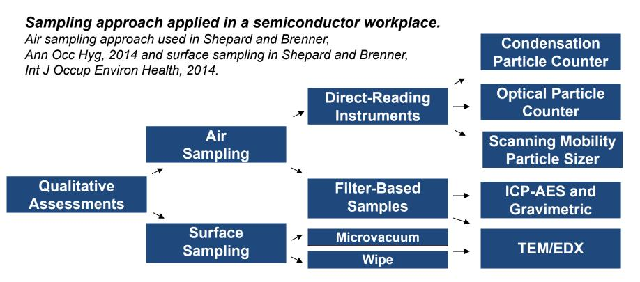
ICP-AES: inductively coupled plasma - atomic emission spectroscopy. TEM/EDX: transmission electron microscopy/energy dispersive x-ray spectroscopy.
