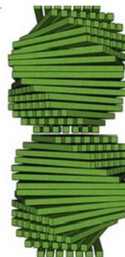
Three-dimensional (3D) model of a Bouligand structure. Image credit: E.P. Chan, NIST.
