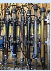
Column filtration system at the Orange County Water District pilot test; the far left column contains the adsorbent. Image credit: Cyclopure.
