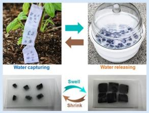
Super moisture absorbent gels that can extract large amounts of water from ambient air, and quickly release it in the form of clean drinking water using only solar energy and enabled by nanostructures in the material. Image credits: University of Texas – Austin.
