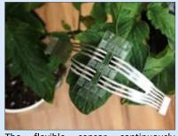
The flexible sensor continuously monitors plants to detect stresses and diseases. Image credit: North Carolina State University.
