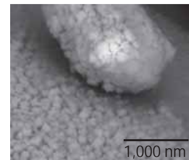
SEM image of silver NPs in a commercial textile
