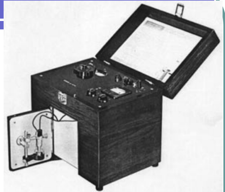
Model G pH meter. Device was closed in wooden box 12" wide by 8" deep by 9" high. - was hardly portable, weighting almost 8 kilograms.
