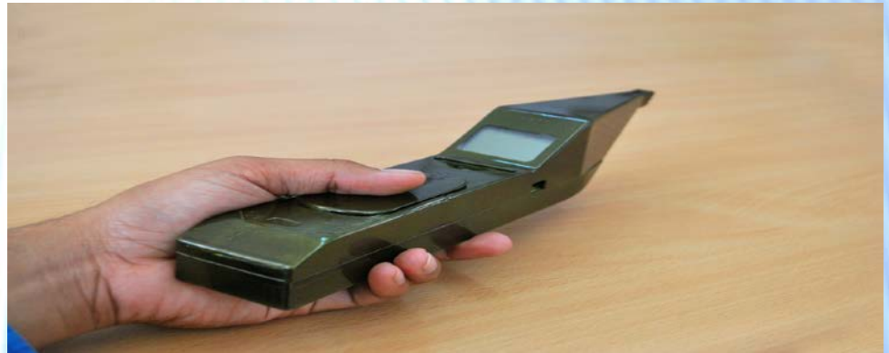
A cantilever based low-cost explosive detector
