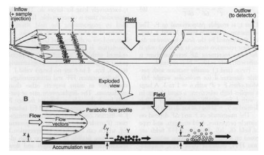
Cross-flow fields separate nanoparticles by size, charge, density, etc.
