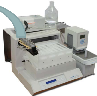
Flow-through diffusion cell System (PermeGear In-Line ILC07)
