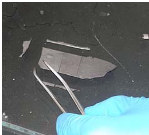
Electrochemical capacitor electrodes from titanium carbide-derived carbon (TiC-CDC). Credit: John Chmiola, Department of Materials Science and Engineering, Drexel University.
