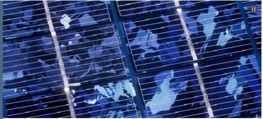
The light glinting off the surface of this solar photovoltaic cell signifies lost efficiency. Scientists are looking to nanotechnology to boost solar power, including by reducing the amount of sunlight that silicon wastes through reflection. (Image: Nat Geo)
