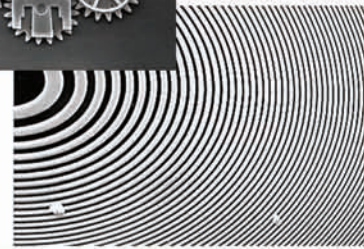
Zone plate X-ray "lens" Outermost ring spacing ~35 nm
