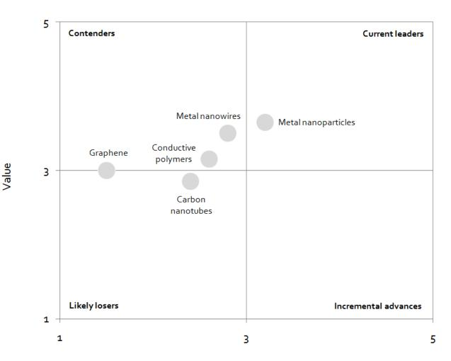
Currently, indium tin oxide (ITO) is the standard transparent conductive film (TCF), but its high cost, vulnerability to shortage or price fluctuations of indium, and brittleness create opportunity for emerging technologies including metal nanoparticles, metal nanowires, and carbon nanotubes (CNTs).
